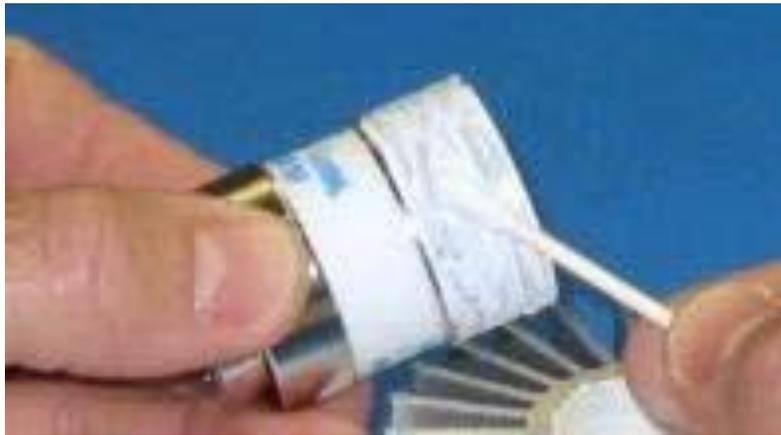
Step 3: Apply a layer of thermal compound to outer bands of the cooling ring and cathode end of the lamp. Take care not to apply compound to the lamp window or ceramic surfaces. Any compound should be removed with the use of alcohol and a clean applicator and/or wipes.
