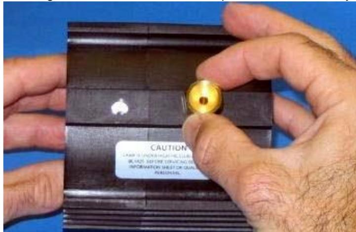
Step 16: Insert brass connectors through housing and into heatsinks. Note that the connector with the larger thread size (10-32) is for the anode/rear heatsink and the smaller thread size (8-32) is for the front/cathode heatsink.
