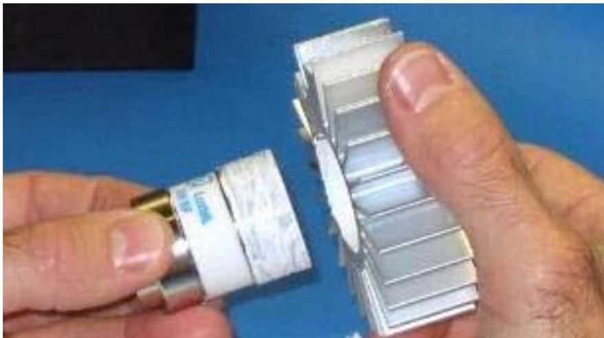
Step 4: Insert front end of lamp assembly with cooling ring into cathode heatsink and rotate until fully inserted.
