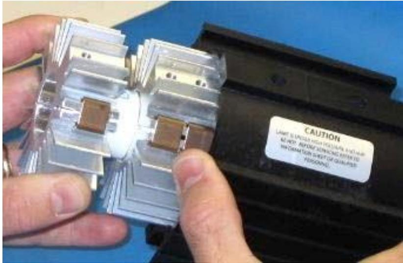
Step 15: Insert the lamp with heatsinks into the housing, assuring that the window/cathode end is facing the housing end with cut-out that holds optional timer assembly.
