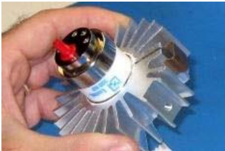
Step 6: Place one spring clip onto slotted area of heat sink.
