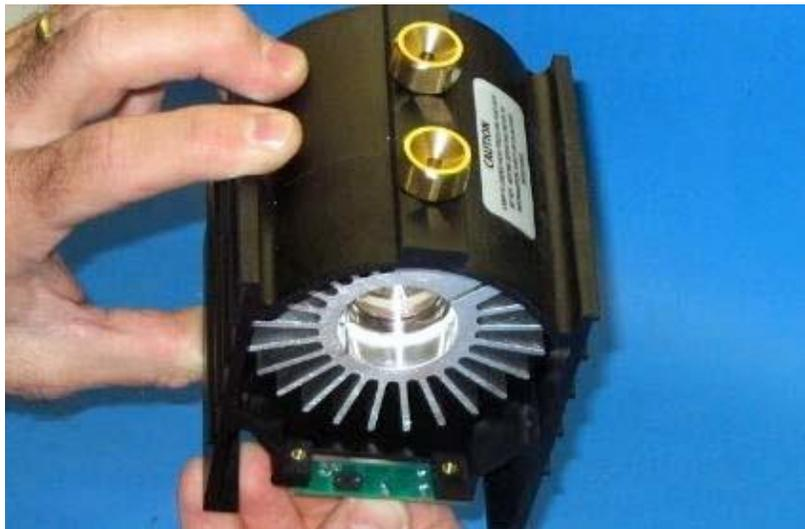
Step 18: If using optional photodiode timer assembly, mount as shown with photodiode facing up and printed circuit board mounted from the bottom. Scaled hour meter is on the opposite side of board.
