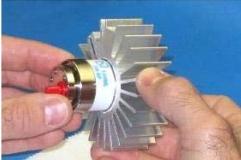
Step 5: Assure the lamp and cooling ring are fully seated into heatsink. Lamp metal band should protrude approximately .040" from heatsink when properly seated. Lamp may be rotated for preferred pinch off orientation at this time.
