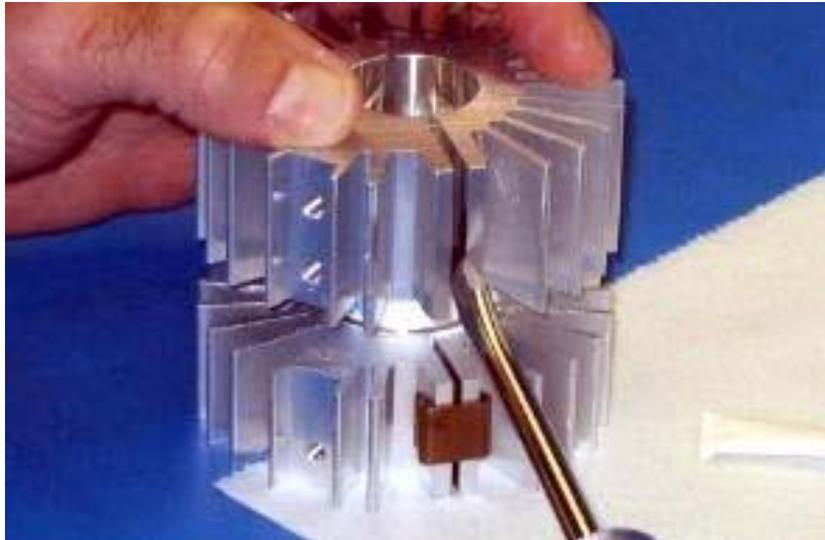
Step 12: If needed, the heatsinks may be pried apart slightly by using a slotted screwdriver. Care should be taken not to force the lamp or deform the heatsinks.
