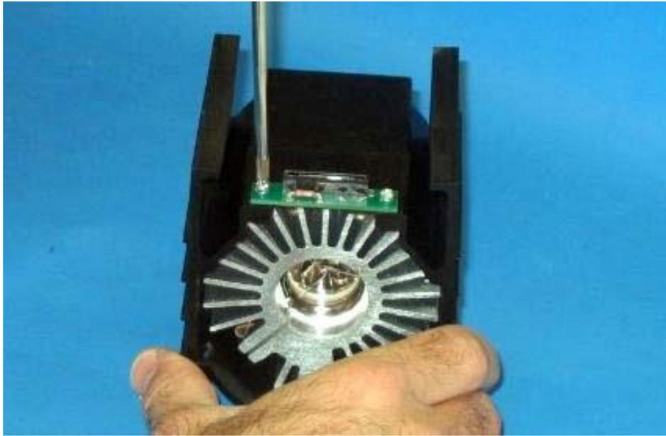
Step 19: Align mounting holes in printed circuit board with threaded inserts in housing and secure with two 4-40 x 1/4" screws.
