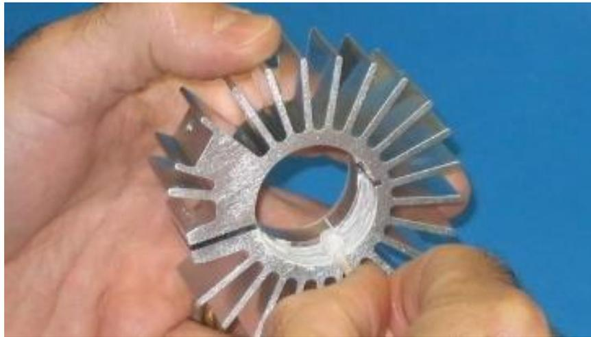
Step 1: Using tip applicator, apply a layer of thermal compound to the inside of the cathode heatsink. The cathode heatsink is 1" thick (25.4mm). Apply compound only to the area where the lamp and cooling ring will contact the area of larger inner diameter. Set cathode heat sink aside.
