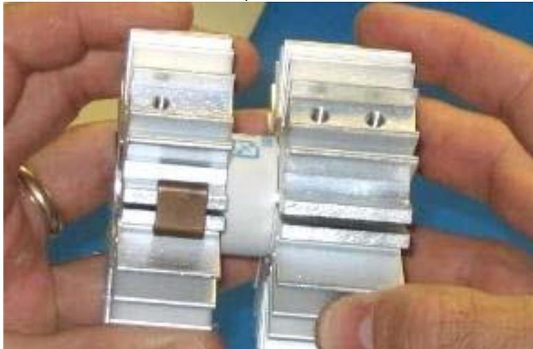
Step 13: Align the slots and threaded holes of both heatsinks by rotating the anode heatsink.
