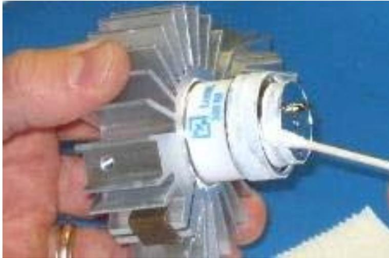
Step 10: Apply compound to the outer band and diameter of anode base. Take care not to damage the pinch off seal.
