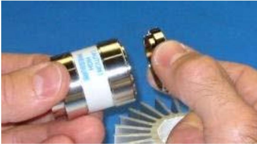
Step 2: Place cooling ring securely onto cathode - front end (window side) of lamp. Assure the cooling ring is seated. If you are using a cooling ring assembly with a filter, take caution not to touch filter with fingers or thermal compound.
