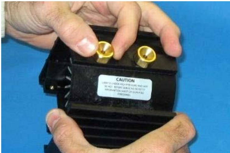
Step 17: Connectors may be secured tightly by hand. If tightened with a wrench, use a torque wrench and do not exceed 16 in-lbs.
