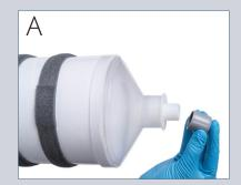
Filter must be installed in housing, and cap removed during testing.
