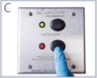
To test Filter. Press "Test Filter" button whilst system in "ON". Test filter at start of each procedure
