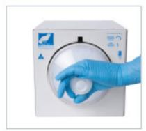
Remove cap to install tubing and replace at end of procedure.
